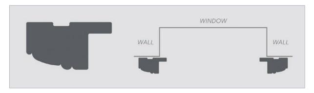
L FRAME Frame fitted onto window or into recess.
