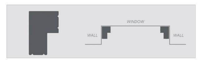
Z FRAME The perfect frame for shutters requiring fixture to the outer edge of the window recess, enabling your shutter panels to open fully and sit against your exterior wall.
